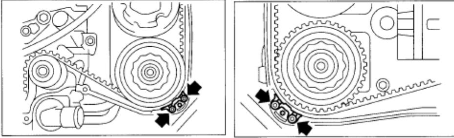
Step 18) Remove Company23 Cam lock.
