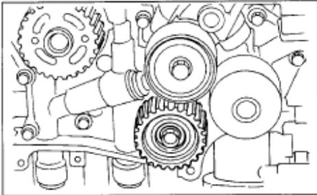
Step 10) Remove the automatic belt tension adjuster.
