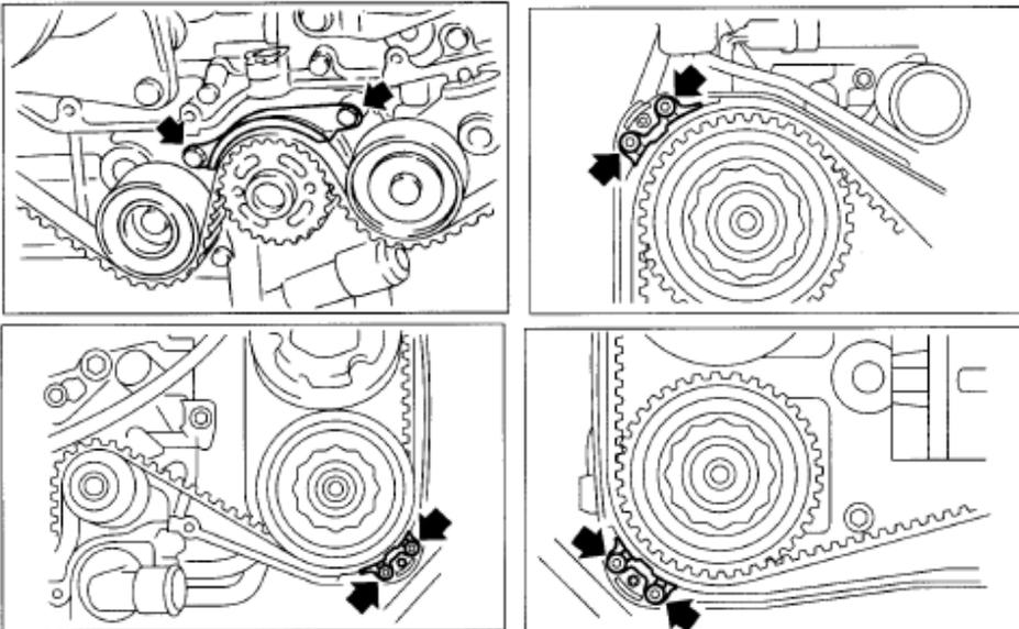
Step 4) Reinstall the crank pulley and crank bolt and turn the engine over to align alignment marks on crankshaft sprocket, left-hand intake camshaft sprocket, left-hand exhaust camshaft sprocket, right-hand intake camshaft sprocket, and right-hand exhaust camshaft sprocket with notches of backside belt cover and cylinder block. You will now need to remove the crankshaft pulley. See Company23 Crank Pulley Instructions.
