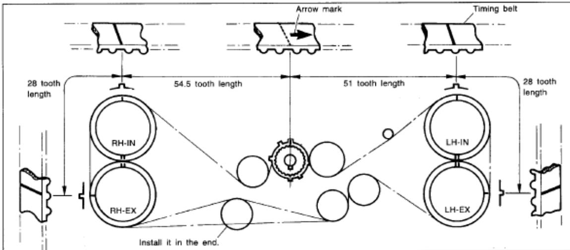
Step 16) Install belt idlers and tighten to 39 Nm (4.0kgf-m, 28.9 ft. lb)
