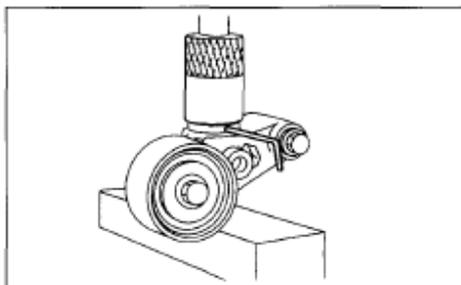
Step 12) Install the tensioner and tighten to 39 Nm (4.0kgf-m, 28.9 ft. lb)
