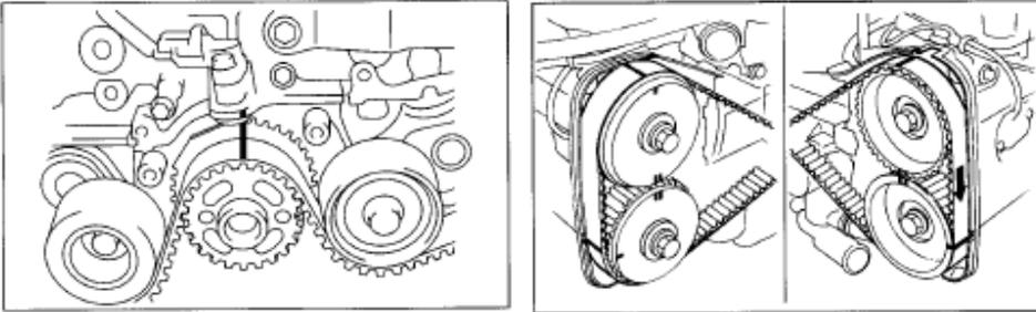
Step 5) For AVCS cam sprockets, remove the cover plates and set aside. Install Company23 Cam lock onto left-hand side exhaust and intake camshaft sprockets. If you have intake AVCS cam sprockets only, install spacer on bottom side of the tool between the hex lock pin and the curved tie bar. The tool should be parallel to the cam pulley surfaces.
