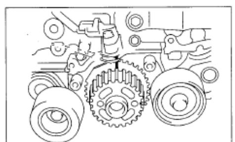
Step 15) Reinstall the timing belt. For reference, verify alignment marks from Step 15. Ensure the belts rotating direction is correct.
