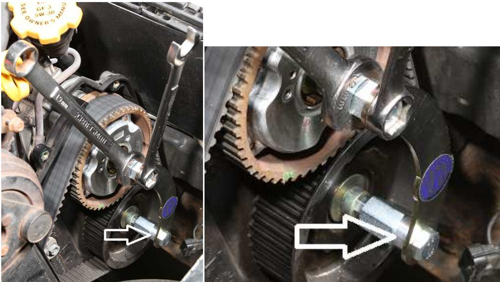
Step 6) Using a 19mm wrench and a 17mm wrench, tighten the top and the bottom cam lock bolt while holding the hex of the hex lock pin. This locks the cam positions so they do not rotate when the belt is removed.
