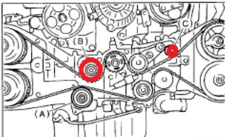
Step 17) Reinstall timing belt guides (manual transmission vehicles). Tighten bolts to 9.8Nm (1.0kgf-m, 7.2 ft-lb)
